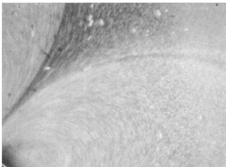
FIG. 10. Secondary roll cells that emerge in the bulk phase, bounce off the interface, and dissipate in the bulk phase.
